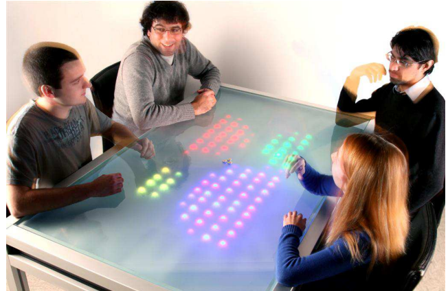
Figure 1. The current design of Reflect with color-coded circles around each speaker position indicating how much the person has spoken.
